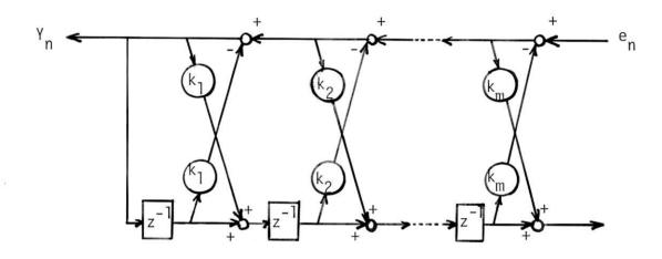
Fig. 2.2.1 Ladder realization of autoregressive process
