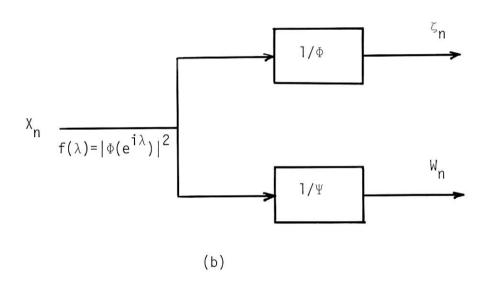
Fig. 4.1.1 Mismatch of an inverse filter
